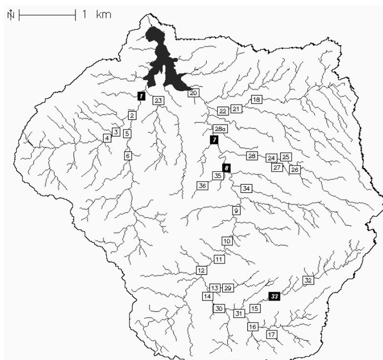
Figure 4. Location of check-dams within the Cárcavo basin (in black the dams where bankfull discharge measurements were carried out) (Source: Castillo et al., submitted).
