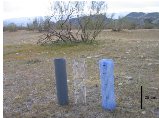
Fig. 1. View of the field site depicting Retama sphaerocarpa shrubs and the three different types of tubes used in this experiment. Left : PVC tube that did not allow root trespassing or water flow; center : Mesh tube that allowed neighbouring roots to get inside the tube and free movement of water; right : Netting tube that did not allow root trespassing into the tube but allowed free transfer of water between soil inside and outside. The field site is dominated by large Retama sphaerocarpa shrubs surrounded by barely vegetated areas. Note the facilitative effect of Retama shrubs on understory plant community compared to gaps between nurse shrubs.
