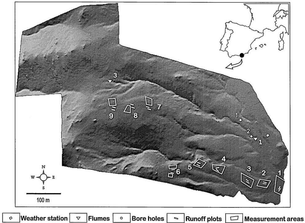
Fig. 1. Experimental layout at the Rambla Honda field site.
