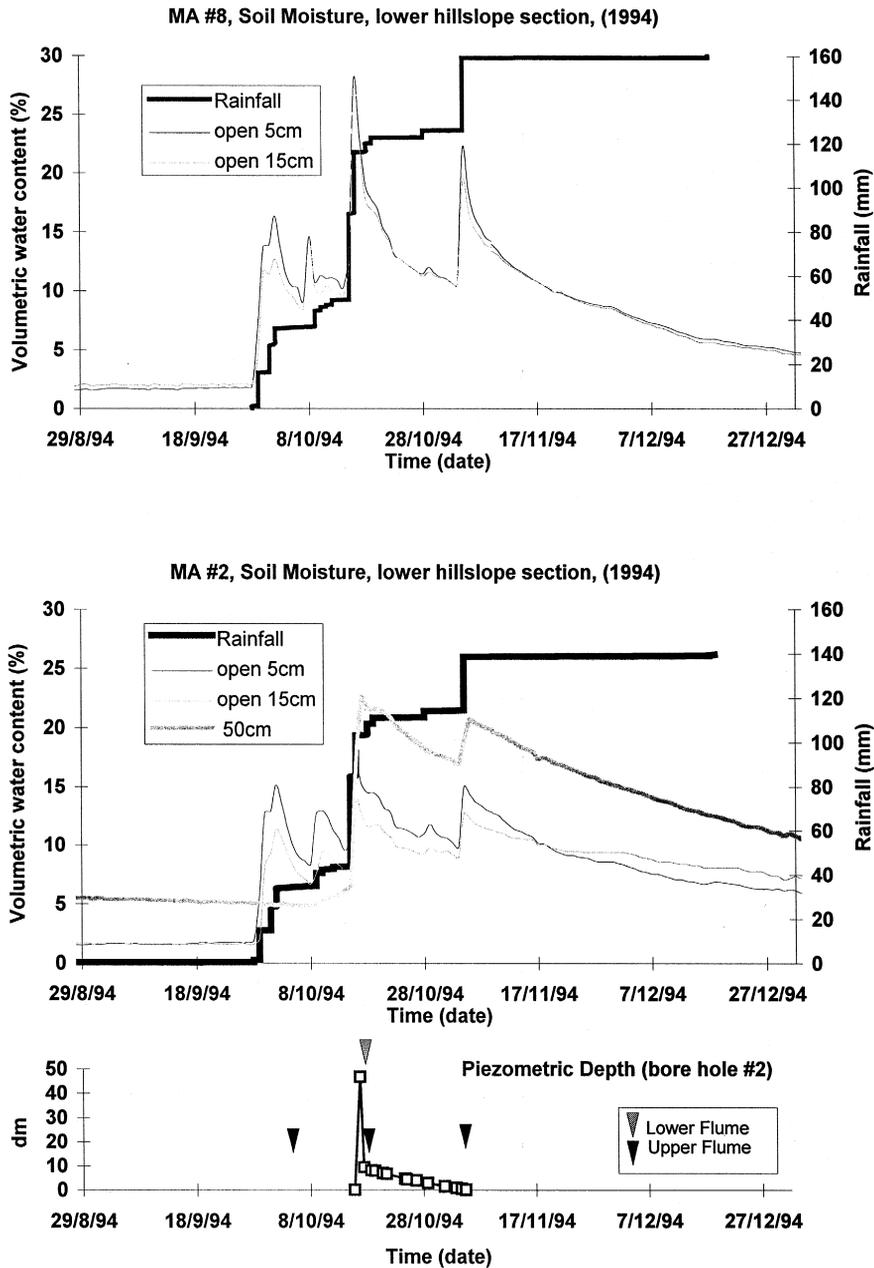
Fig. 4. Cumulative time evolution of rainfall and soil moisture, in bare ground (open) areas, at 5 cm and 15 cm depth, during the rain period of autumn 1994, at the hillslope sector (MA 8) and the lower fan sector (MA 2) of Rambla Honda. The phreatic level records are next to the lower flume and times when discharge was recorded at the flumes are indicated.
