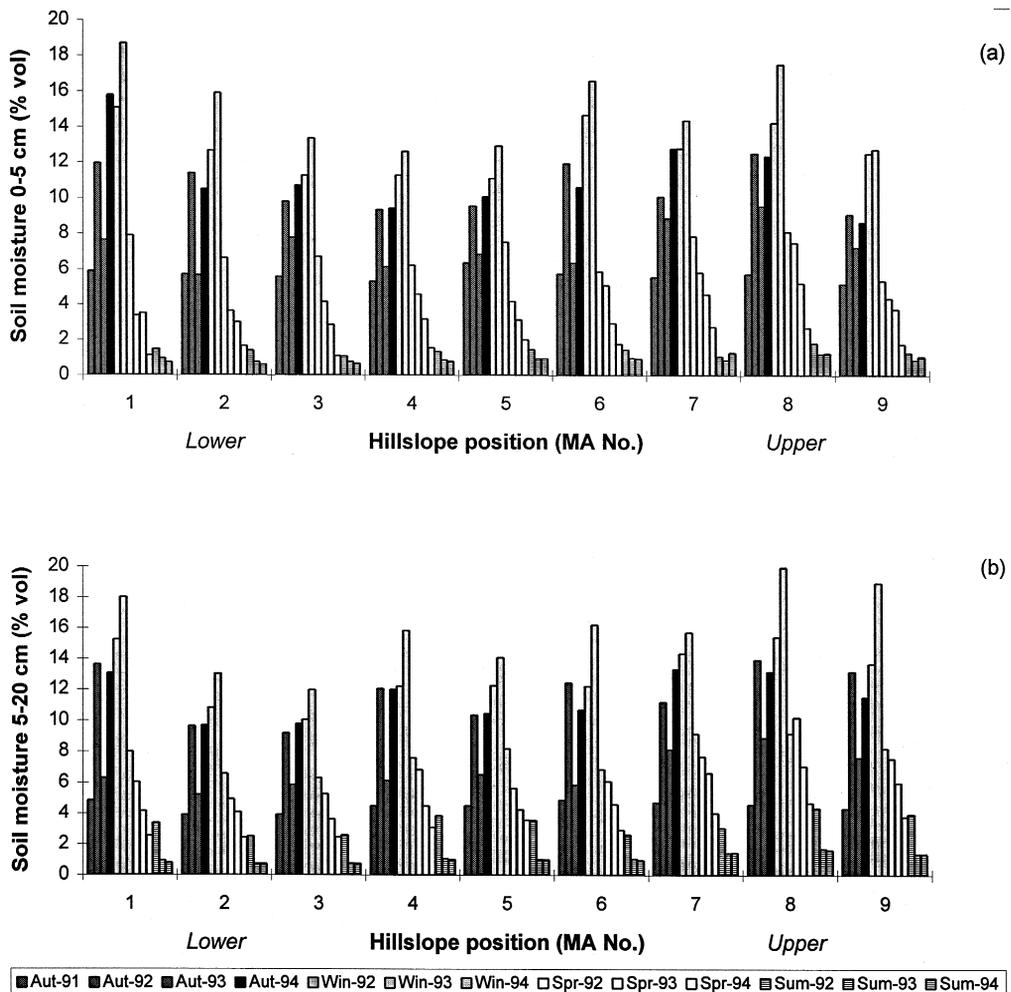
Fig. 3. Mean seasonal soil moisture distribution along the Rambla Honda catena in the study period. (a) 0–5 cm; (b) 5–20 cm. MA 1 to MA 5: footslope sediment fill; MA 6 to MA 9: rocky upper slope. The solid bar shows the soil moisture in autumn 1994, when the reported case study was carried out.
