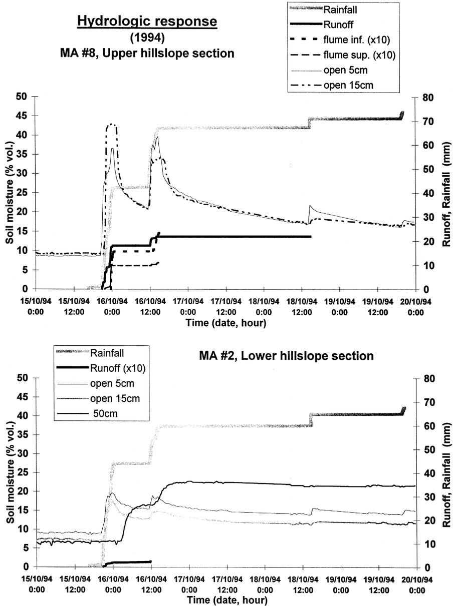
Fig. 5. The same as Fig. 4, but focusing on the period 15–20 October 1994 and adding information about overland flow in runoff plots (2 m × 10 m) and discharge at the flumes.
