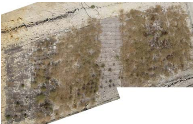
Figure 4. Plots on marly substrate after one year after the plantation. No cover of opportunistic species is observed on plots with no organic amendments (4 th and 8 th plots starting from the right).
