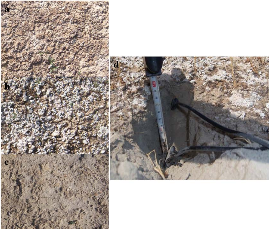
Fig. 1. Picture of the different types of surfaces: a) cyanobacterial BSC, b) lichen BSC and c) BSC-scraped soil (six months after BSC removal), and installation of the moisture probes in the soil, at 0.03 and 0.10 m soil depths (d).
